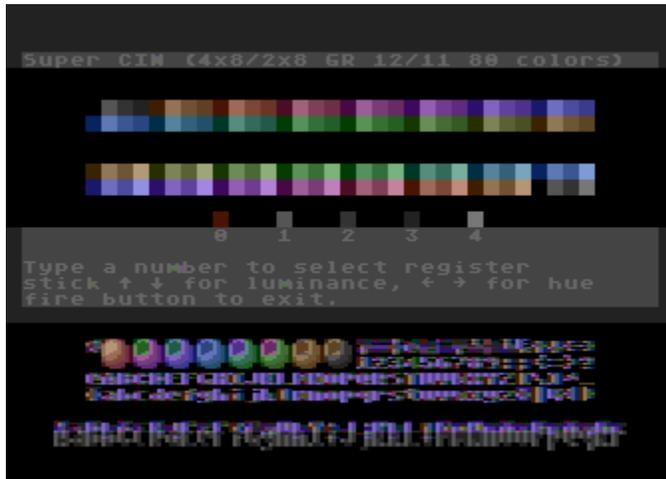
This is a modification of the CIN 12 mode. A display list shift from Antic 4 to Graphics 0 combined with a GTIA shift to Graphics 11 increases the color resolution to 80 colors onscreen at once at ANTIC 4 resolution. This mode is unusable in ANTIC 5 (40x12).
