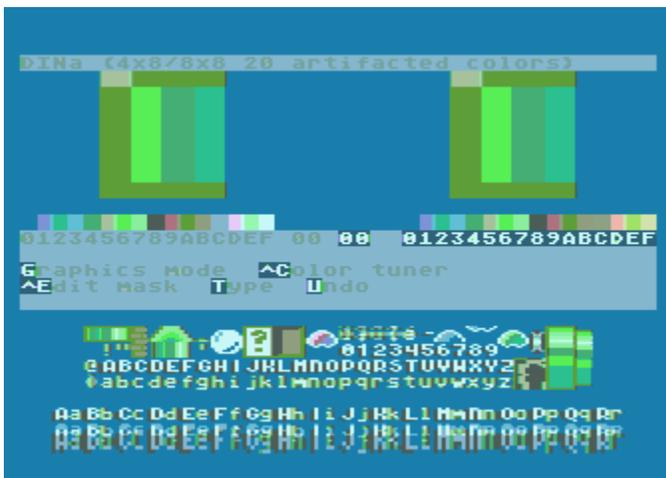
This display mode flips between two display lists stored in memory: Graphics 0 and ANTIC 4 (Graphics 12). The pixel resolution is 320 across, in an 8x8 character grid, but 10 colors can be displayed onscreen
