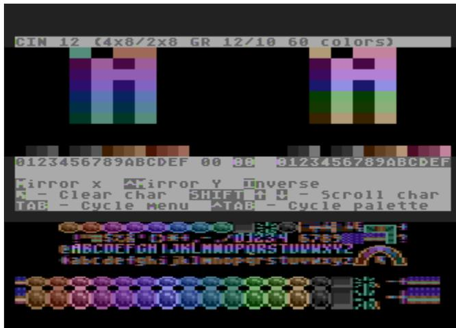
This is one of the most useful CIN modes. An ANTIC 4/5 display list is used and the GTIA is flipped between normal and Graphics 11. 36 colors can be used per character grid, with the usage of inverse characters bringing the total color resolution to 60 colors. Although not required, it is good practice to use monochrome colors for registers 708–711, which interface with the 14 hues accessible in this mode
