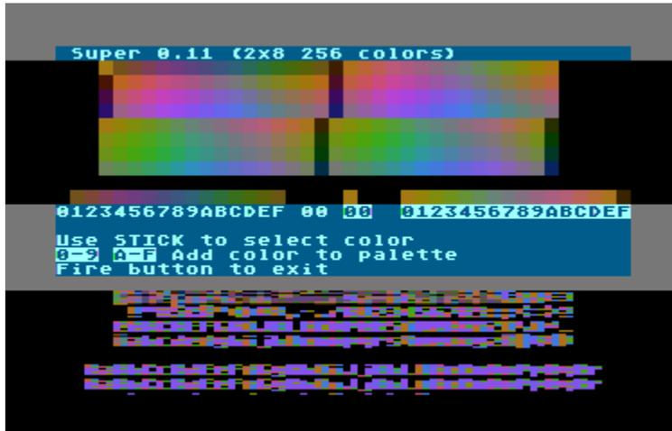
This is based off of Graphics 11, the 16 chroma mode. By flipping character sets and register 712 (which controls the luminance of the colors) a total of 256 colors at three luminances can be seen.
