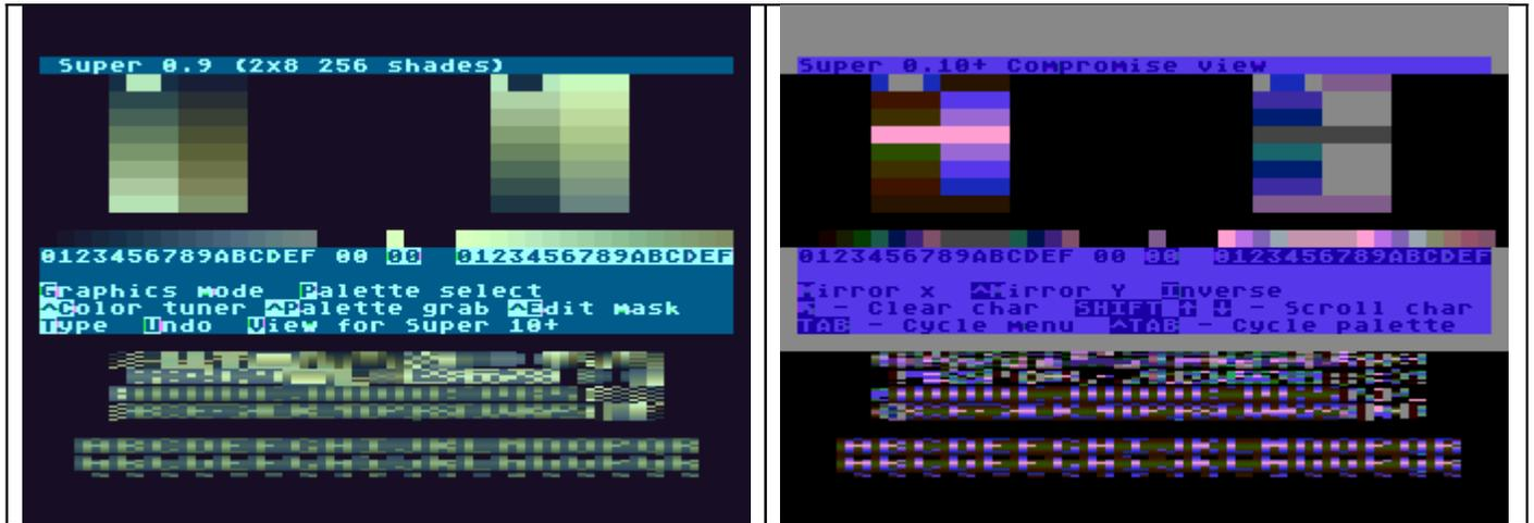
Each pixel on the grid can hold any of 256 color values. In modes based on Graphics 10 (Super 10, Super 10+, HIP 0 and CHIP 0) some of these colors will be redundant. Also, in Super 10, you can use identical color pairs in a dithering pattern similar to Super IRG
