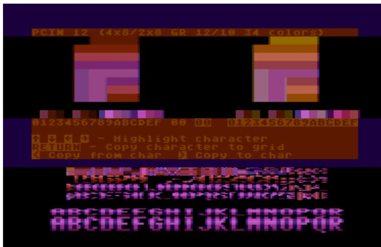
This mode shifts the GTIA into Graphics 10, the paletted mode. The colors are controlled from registers 705–711 and a total of 34 colors can be perceived onscreen at once.
