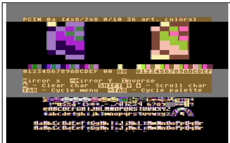
These three display modes mix a Graphics 0 screen with one of the GTIA settings. The result is a 2x8 GTIA character grid, which can also display 4 Graphics 0 pixels. 18 to 32 colors can be seen onscreen at Graphics 0 resolution, and this number is doubled when Graphics 0 artifacting is taken into account.
