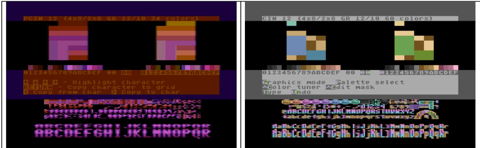
The Antic 4 data occupies a 4x8 grid, but as this mode is paired with a GTIA mode, this means that the GTIA color data will automatically occupy a 2x8 space on the grid. For example, in the CIN 12 grid above you will notice that while each 4x8 pixel is a monochrome value, every two pixels shares the same chroma value which is derived from the GTIA overlay.
