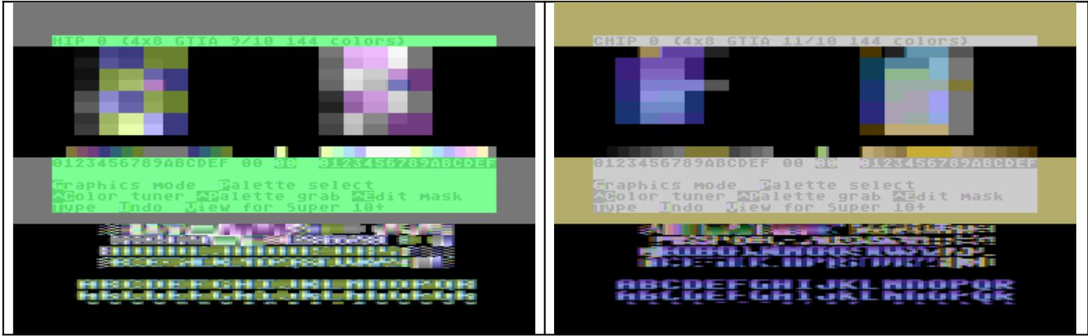
In this case, the mode 10 mask has been shifted to the right. You are still editing in only 2 columns (as in the other GTIA modes) but the pixel you plot will affect the properties of pixels in neighboring columns on the display.
