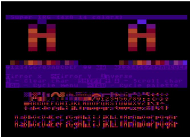
This display mode was used in Bill Kendrick's Gem Drop game. It is based out of an ANTIC 4/5 (Graphics 12/13) display and a 4x8 character grid. The character set is flipped every VBLANK, allowing for 10 colors to be displayed in each character grid. Using inverse characters allows for an extra 4 colors, allowing for a total of 14 colors onscreen at once.
