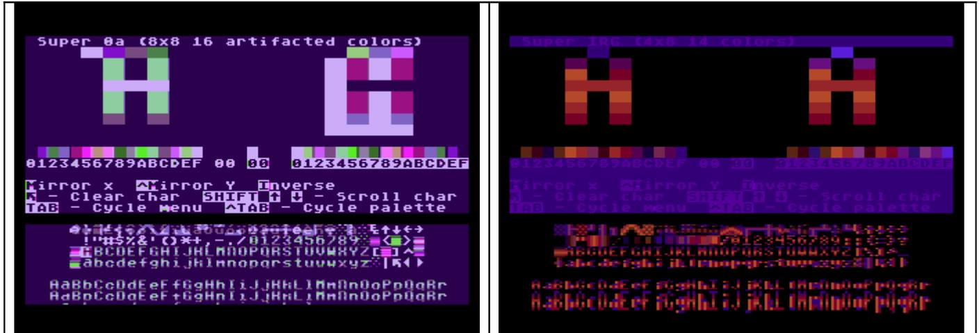
Each pixel on the grid can contain any of 16 colors, although some colors will be redundant. Some colors are different on the inverse palette, and in addition, identical color pairs in Super IRG can be offset from each other to create a dithering pattern to reduce flicker.
